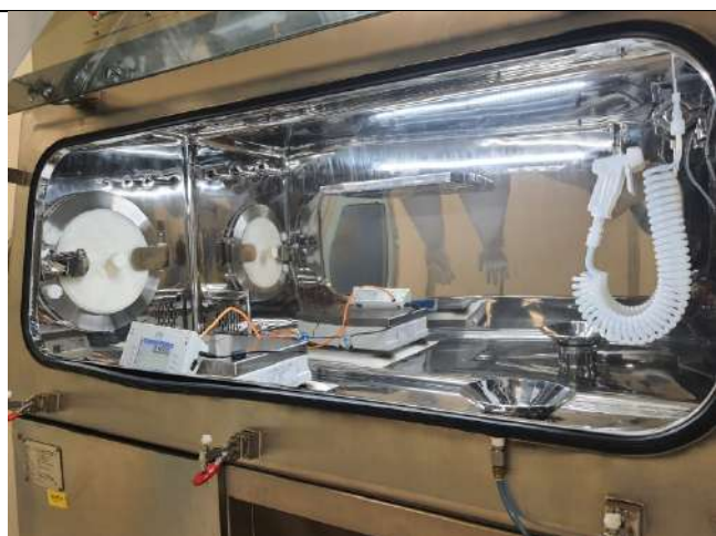
Supplied, installed, commissioned and calibrated sampling isolator
