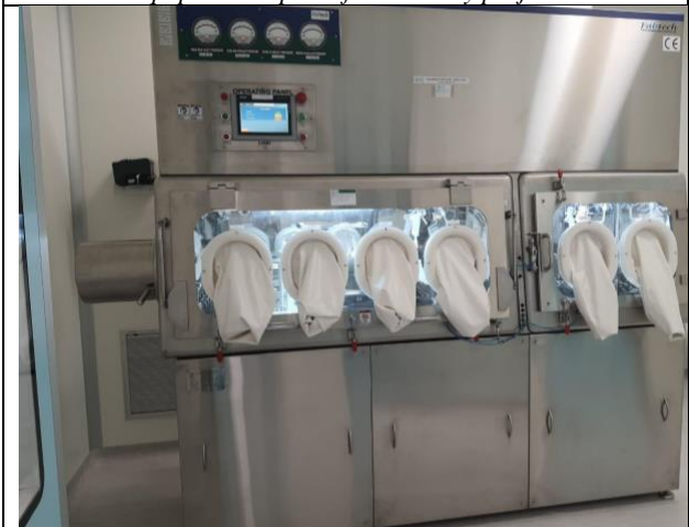
Supplied, installed, commissioned and calibrated dispensing isolator
